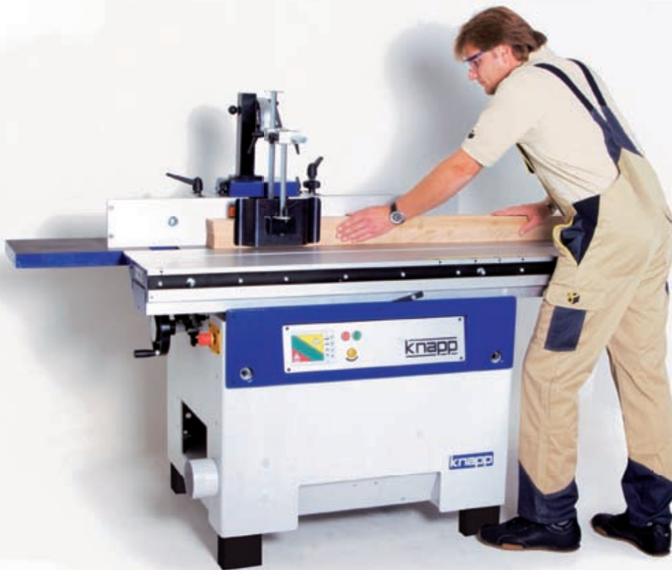
KFS 15 - Circular saw / shaper with sliding table 1500 mm
